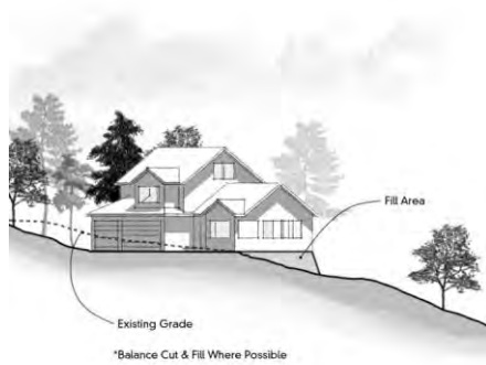
FIGURE 24-17: BUILDINGS DESIGNED TO LIMIT GRADING
