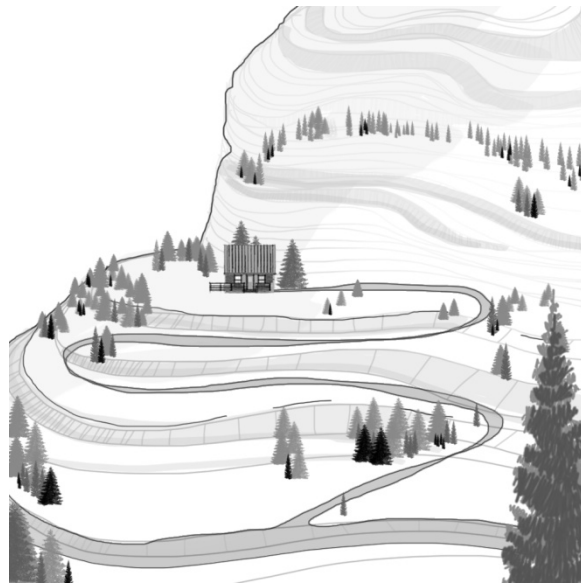
FIGURE 19.72.6: RECOMMENDED ACCESS ROUTE CONFIGURATION
