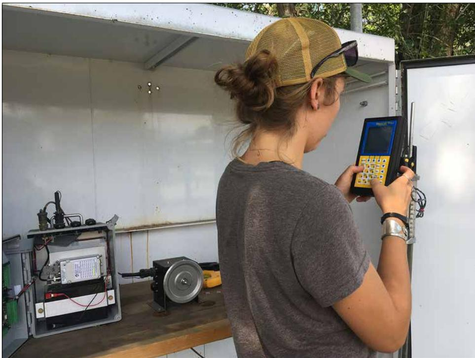
Watershed Program hydrologic technician comparing flow measurements taken in the creek to the most up-to-date rating curves (gage at 300 West on Little Cottonwood Creek).
