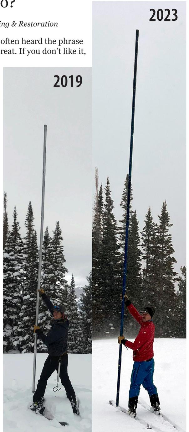
Hollow tubes are used to measure snowpack depth and density up Big and Little Cottonwood Canyons. We broke out our longest tubes yet in 2023!
