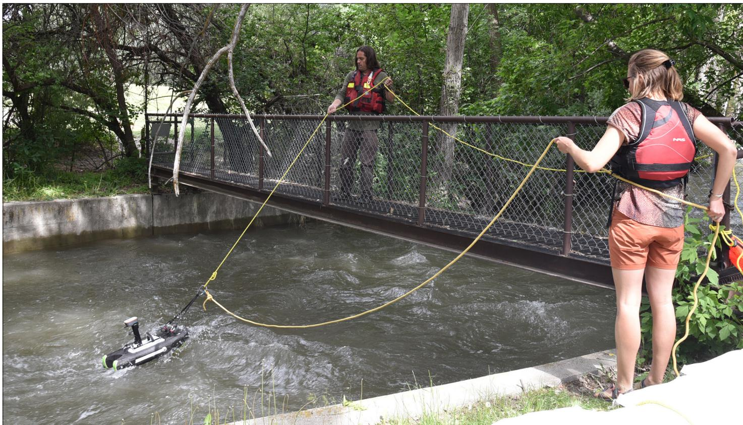
Christened "Tiny Dancer", this little boat uses modern electronics in a compact, portable, and lightweight package to easily and accurately measure river and stream flows from the safety of the shore.
